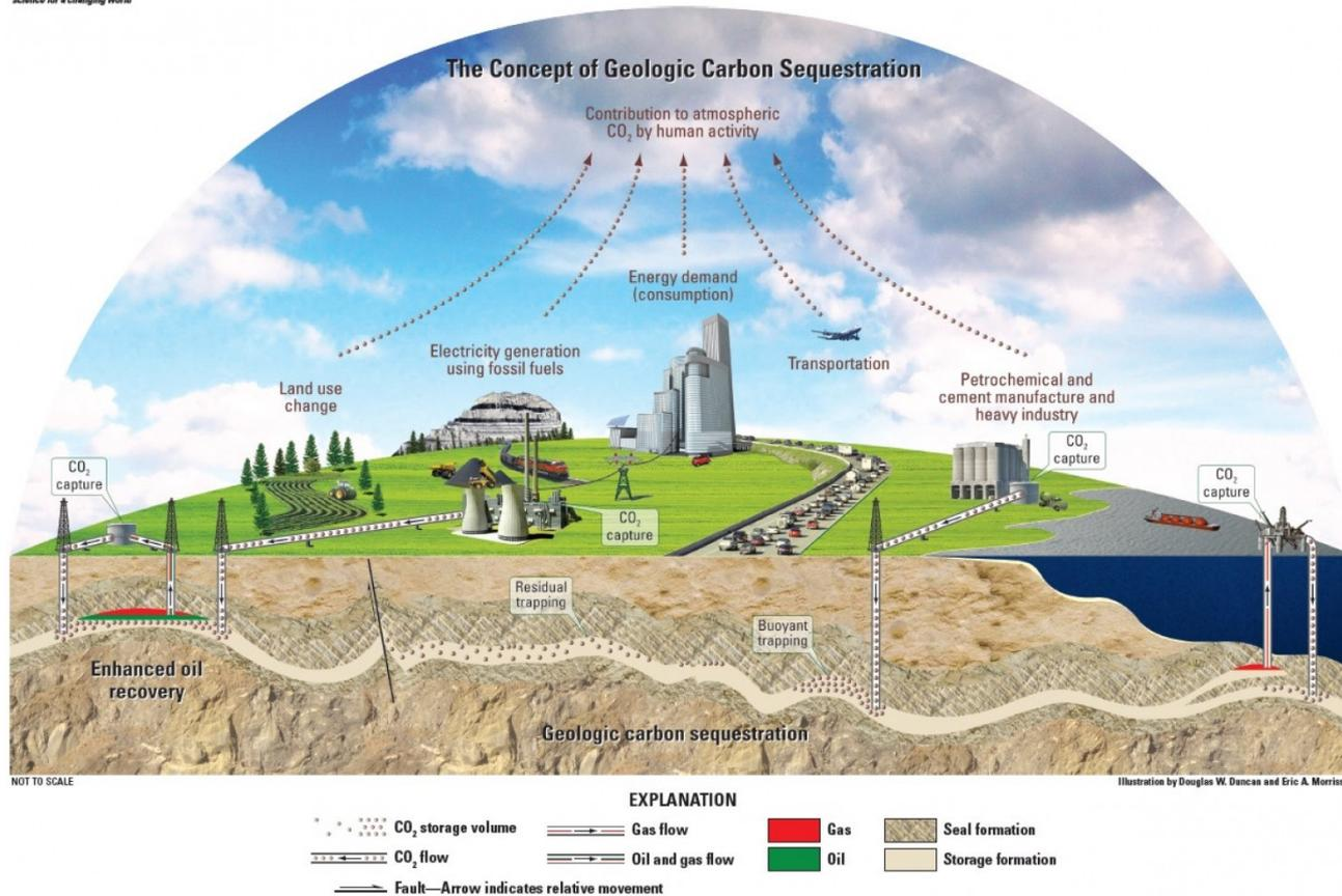
The process of storing carbon dioxide (CO<sub>2</sub>) in underground geologic formations. The CO<sub>2</sub> is usually pressurized until it becomes a liquid, and then it is injected into porous rock formations in geologic basins.
